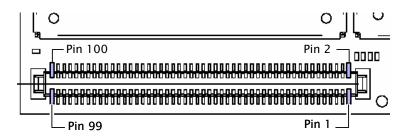
Figure 5.1-1 Wireless modem, viewed from underneath
